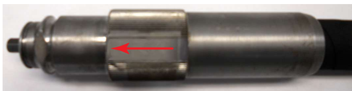
Figure 3: Casing arrow location
